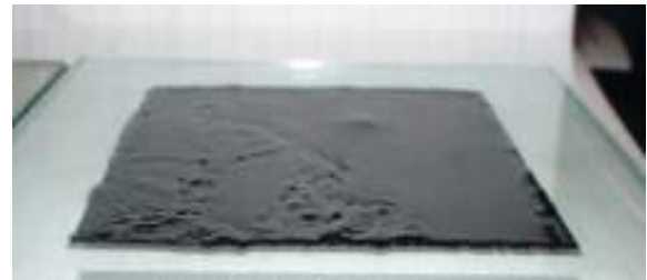
Figure 2. Terminal Blend Binder
